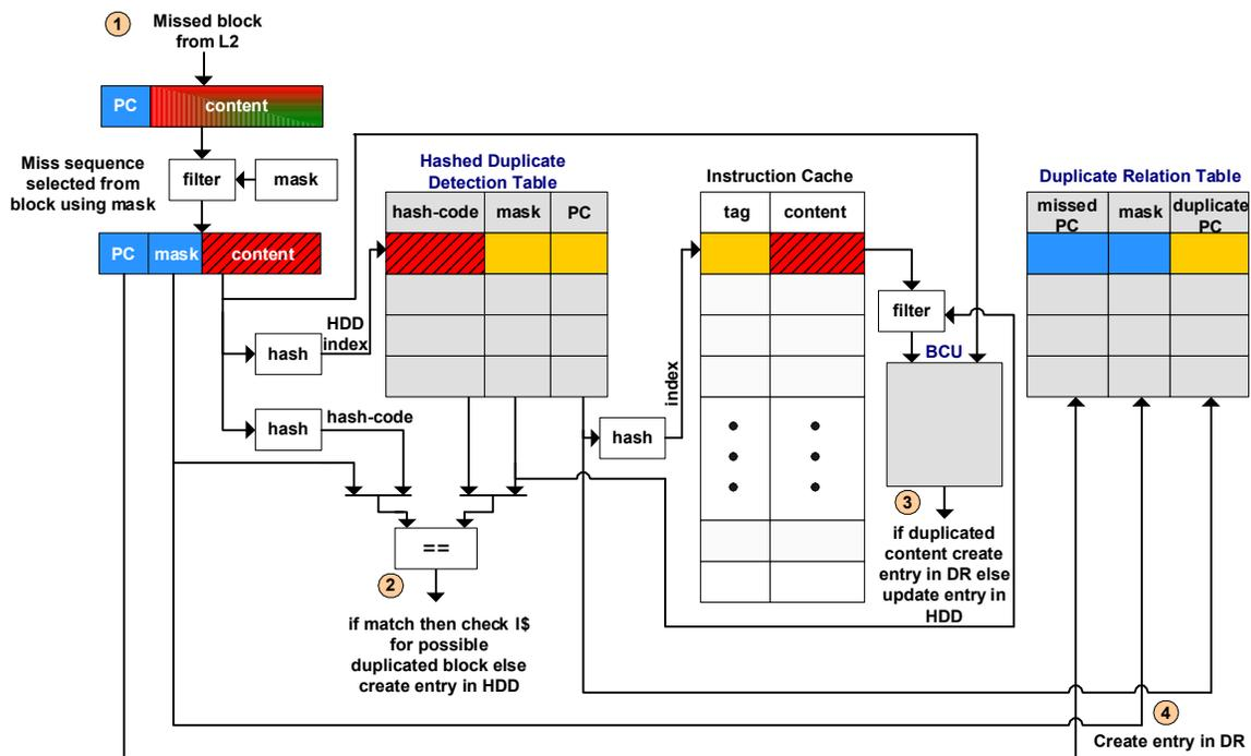
Figure 11. The flow with CATCH for a Cache miss, DR miss and HDD hit
