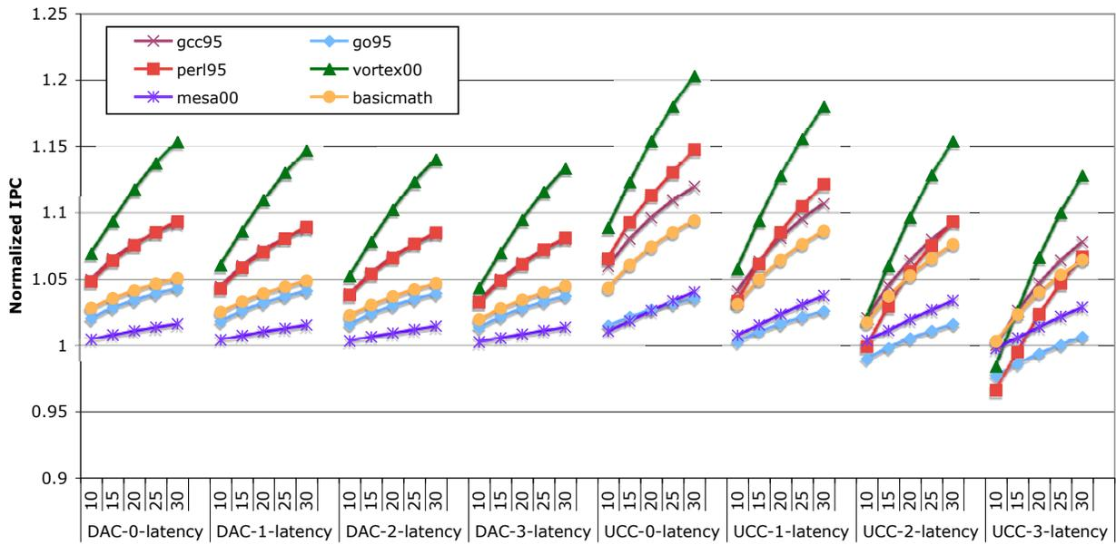
**Figure 9. Performance potential of DAC and UCC for a 2-way, 16KB, 8 instructions per block, instruction cache, for valid blocks (Normalized IPC)**
