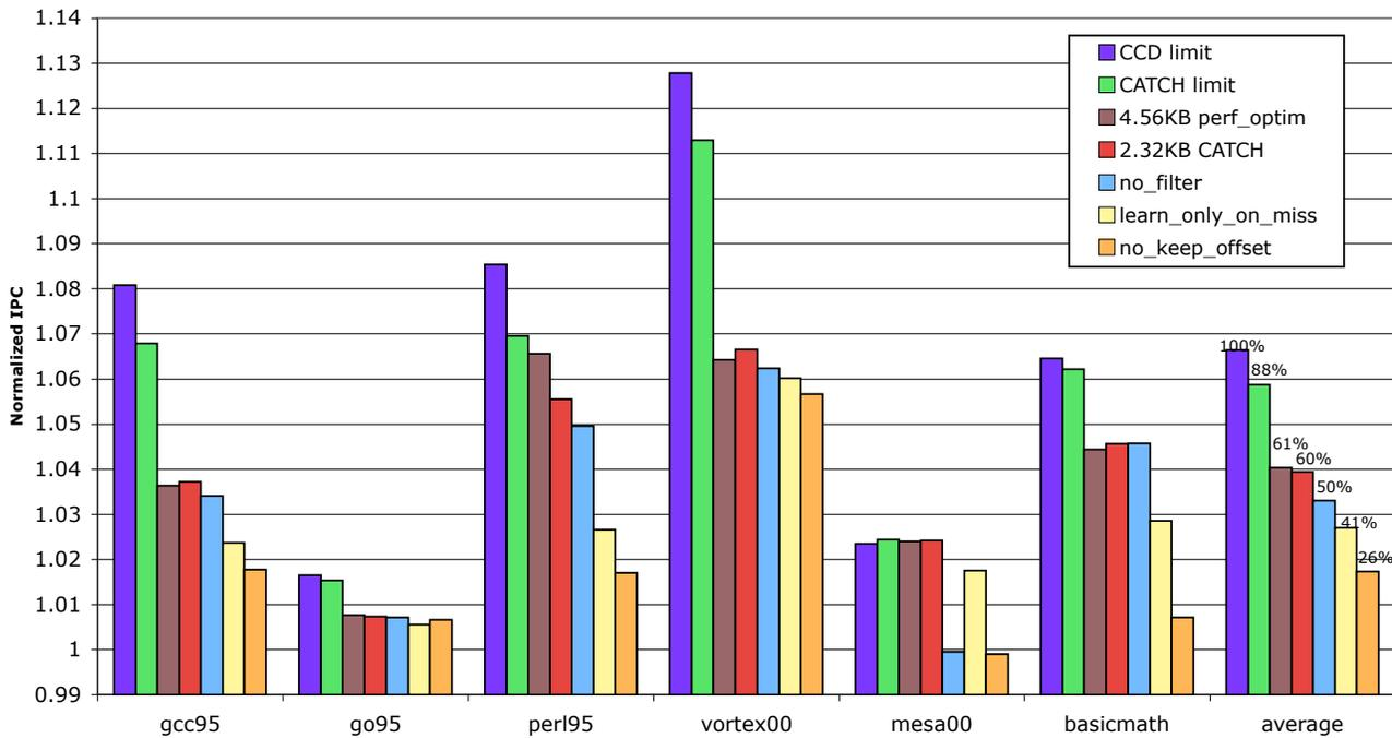
**Figure 13. Effects of applying different policies on CATCH performance**
