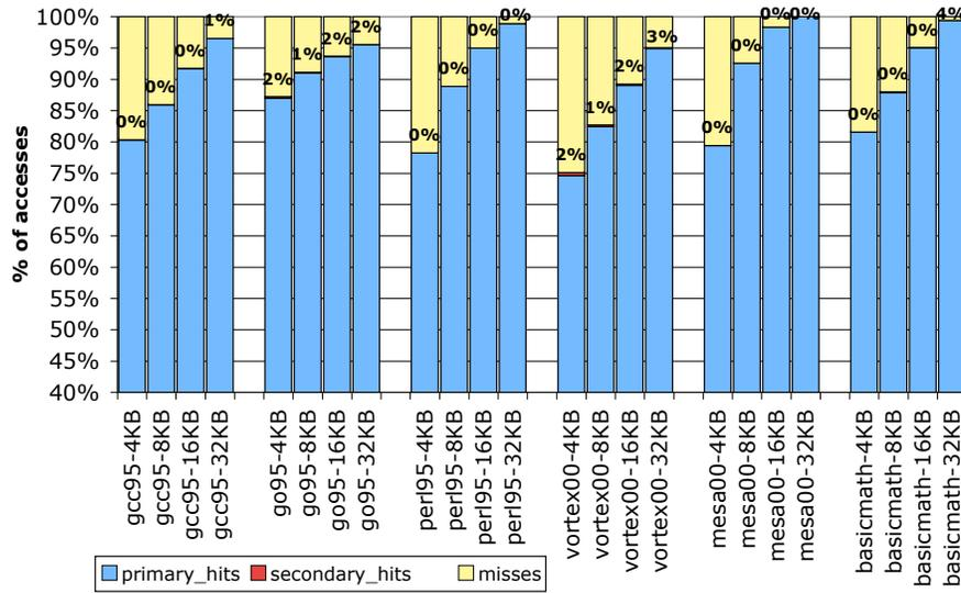
**Figure 2. CCD for a 2-way, 8 instructions per block, instruction cache, for entire blocks**
